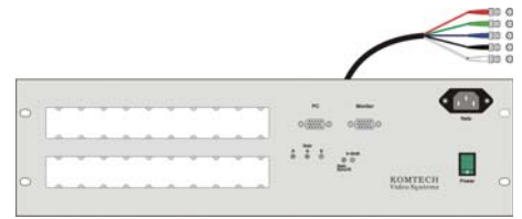
Wall connector panel with VGA interface 2x24TE
